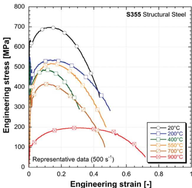
**Project type:** Behaviour of structural steels under fire in a wide range of strain rates
